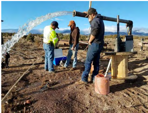
Figure 2 - Pine Valley aquifer testing (Photo: St. George News, 2017 with photo provided by CICWCD)
